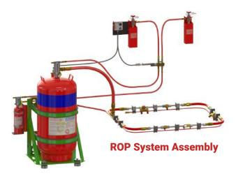
With the use of a distribution network of hoses and stainless steel tubes, the systems deliver the Fire Fighting Agent to the nozzles, with nitrogen gas at 1,350kPa and the concentrate with potable water.
